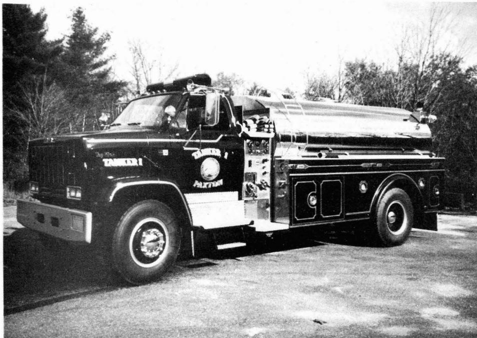
Fire Department's new tank truck holds 1200 gallons of water.
